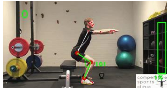
Fig.3. The figure illustrates the computational pipeline for real-time stand-sit movement detection and feedback in the proposed computer vision-based exercise tracking system.
