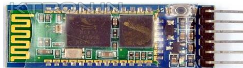
Figure 3: HC-05 Bluetooth Model The HC-05 Bluetooth module is a valuable tool for wireless communication projects, offering a reliable and efficient way to connect devices over short distances. Its compact size, low power consumption, and ease of use make it a popular choice for hobbyists and professionals alike.
