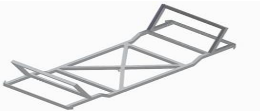
Figure 2: Design of chassis with x type cross section. Fig 2 shows the design of chassis with the x type cross section where the section of the base are connected with each other in x form where the one end of the chassis is connected to another with x form and this design is also safe and we can use it for construction. The Fig 2 design is made in software called solid works and the figure 3 design is made in a software called Catia, All the design which are made for chassis is first
