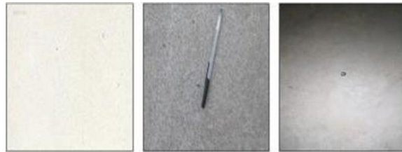
Fig. 2. The provided images depict FOD objects under different light-level categories in FOD-A. Specifically, the left image represents an example of a bright condition, the middle image depicts a dim condition, and the right image shows a dark condition.
