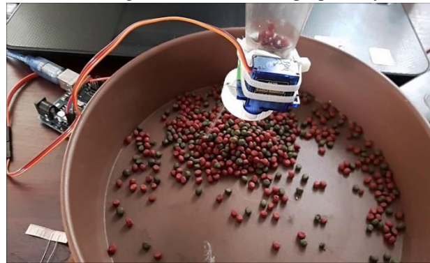
fig .3 shows the dispence of food after command or timer set through Blynk App. It is used to remind the owner to feed the Fish at the appropriate times.
