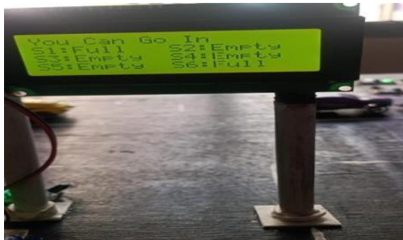
Figure-3 Implementation of slots in Automated parking system
