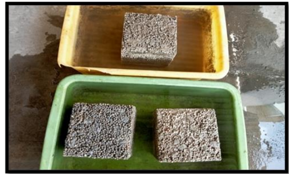
Fig 6: Water absorption test of EPS beads concrete
