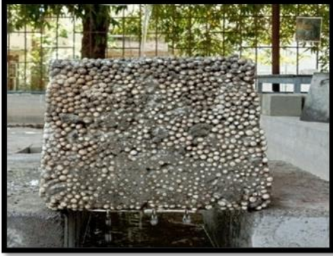
Fig 7: Volume of permeable pore voids test of EPS beads concrete
