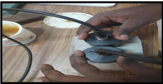
Fig 5: Ultrasonic pulse velocity test of EPS beads concrete
