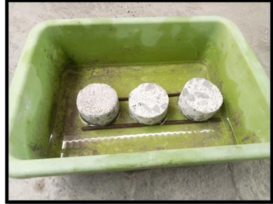
Fig 8: Sorptivity test of EPS beads concrete
