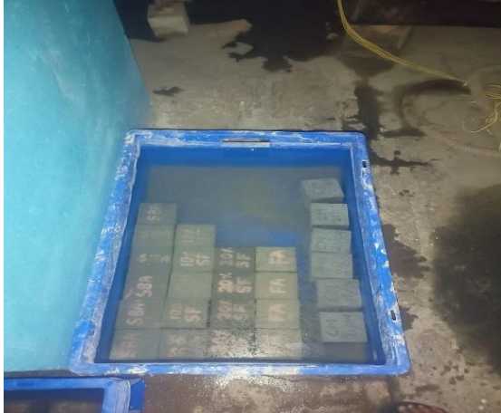
Fig 2. Curing of mortar cubes
