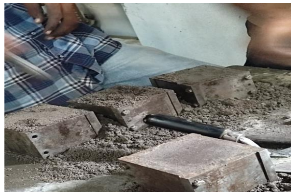
Fig 1. Casting of mortar cubes
