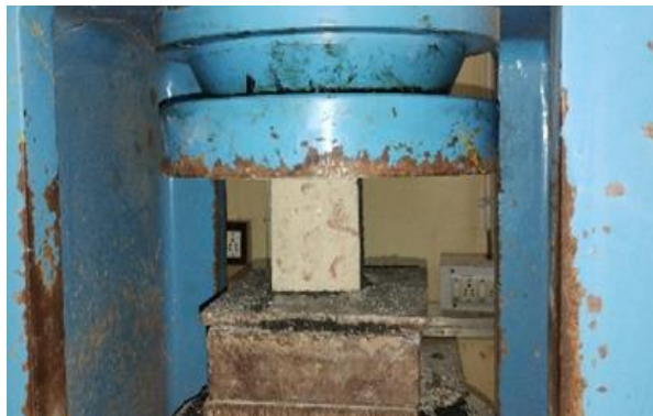
Fig.2 Compressive strength of motar cube
