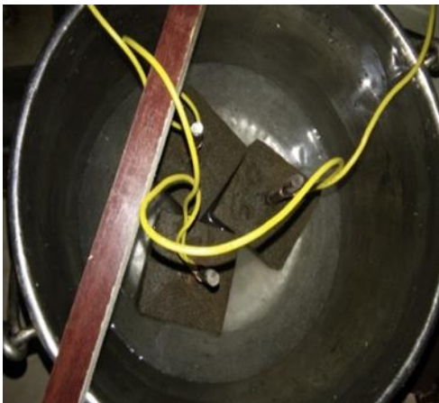
Fig 7 Set-up for Electrochemical Treatment and Steel Corrosion Test on Mortar
