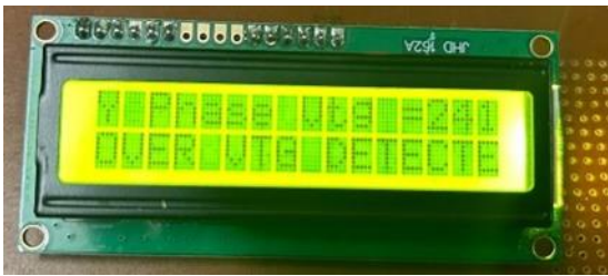
Fig. 8. Over Voltage Fault Detection
