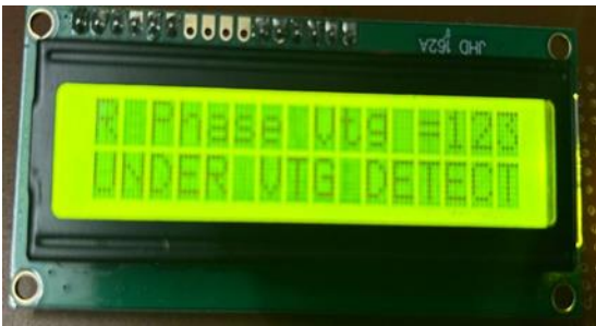
Fig. 9. Under Voltage Fault Detection
