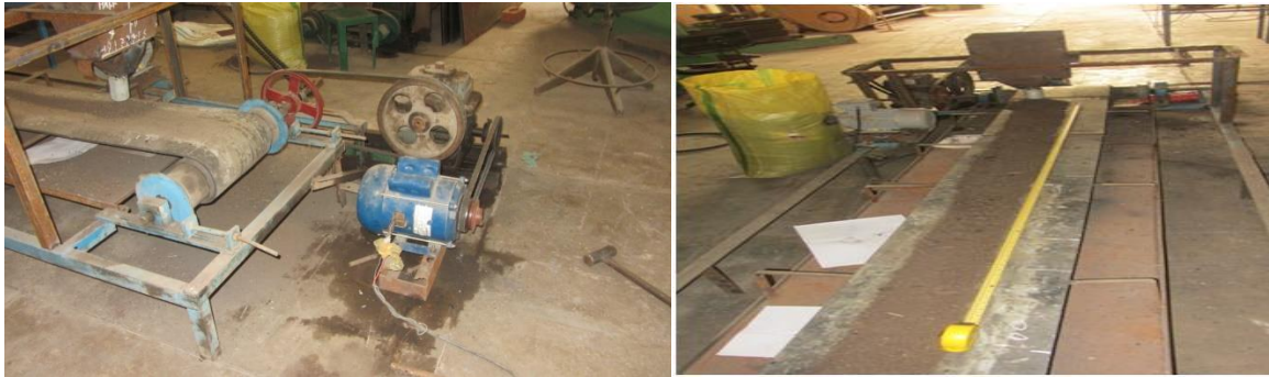
Fig 6. Measurement of distance between seed drop from prototype model by measuring tape
