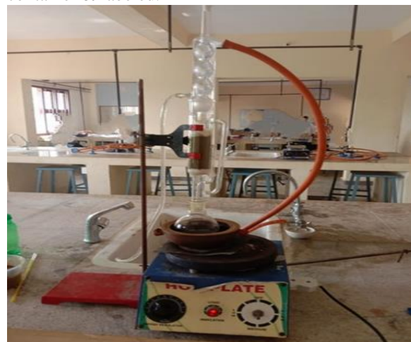
Fig 4: Soxhlet apparatus for the extraction of Murraya koenigii leaf extract
