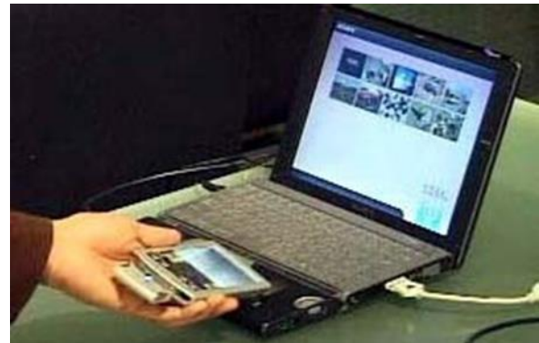
Figure 5: Notebook PC configuration: The RFID reader is embedded at the palm rest.
