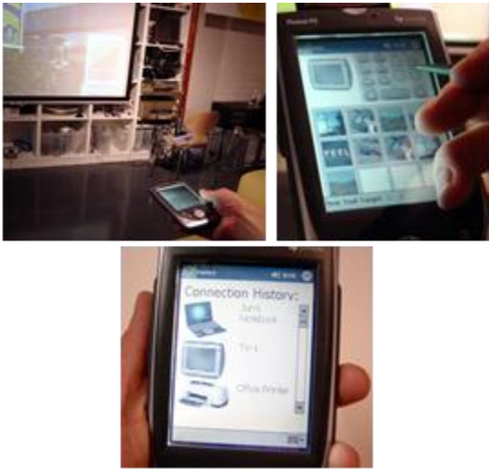
Figure 7: PDA automatically becomes remote commander of target device. (left) An IP address is transmitted from PDA to target device via an infrared beam. (right) The target device responds to the PDA with a description of the device, and user can control it using the PDA. (bottom) The PDA also maintains the access log so user can also connect to the device through the "recently connected" list.
