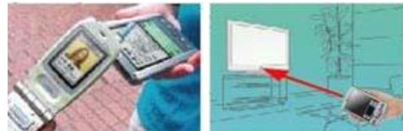
Figure 2: Two typical operation styles of proximal interaction. (left: two devices within close proximity, right: beaming at target device)
