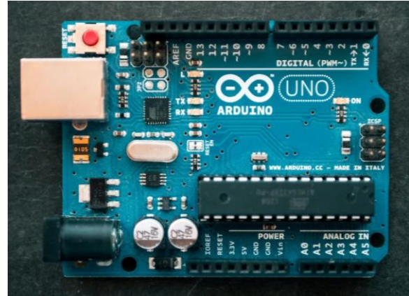
Fig : 3 Atmega328P is a single-chip microcontroller The captured data are displayed on the display unit and then transported to the local server for broaden administering, storing, and investigation purpose. Figure 4 shows the assembled prototype.
