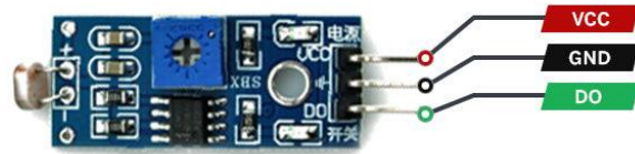
Fig. 6. LDR Sensor Pin Configuration
