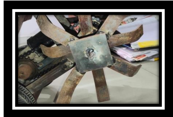
Fig 2: J Shaped Cutting Blade
