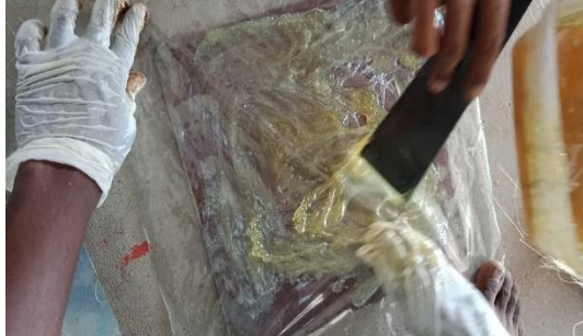
Fig. 4. Hand Layup Process
