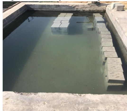
Figure 4.2(b): Concrete Cube in Curing Condition
