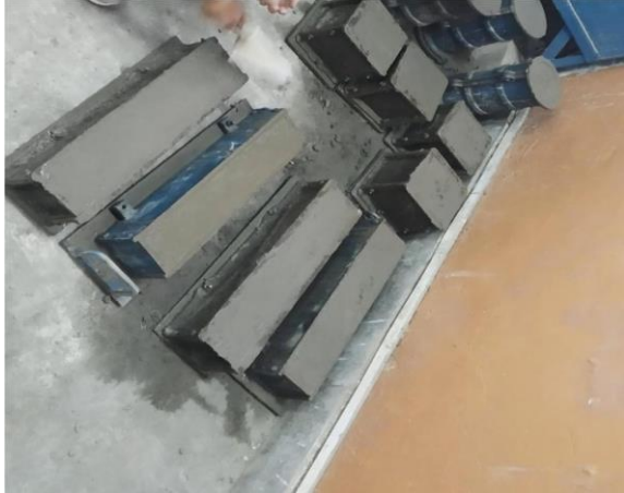
Figure 4.1: Casting of Beams and Cubes
