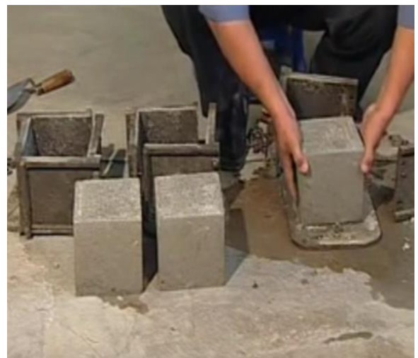
Figure 7Concrete cube casting
