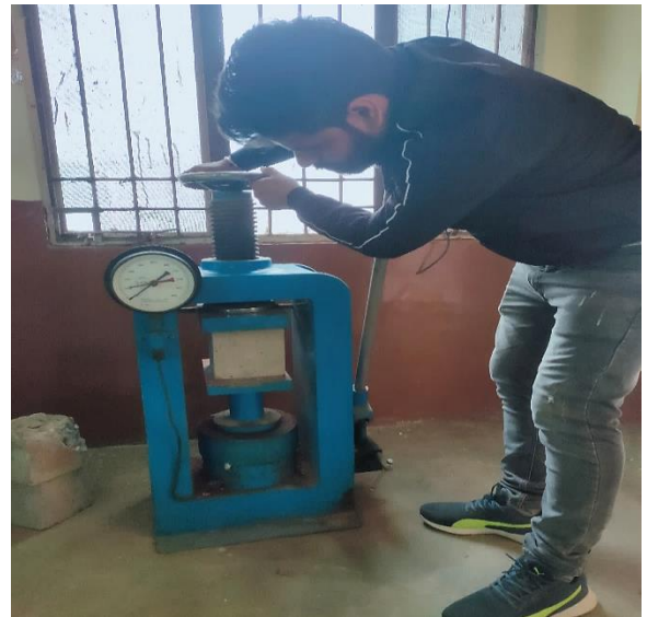
Figure 6Concrete cube Compressive Strength testing
