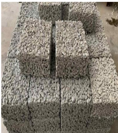
a) No-Fines Concrete
