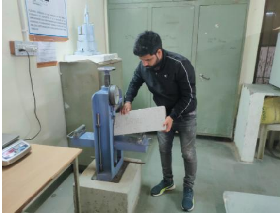
Figure 8 Concrete beam flexural strength testing
