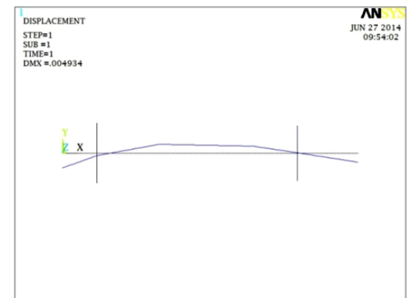
Fig. 4.9 Deflection at the spindle nose for NSK bearings (heavy preload)
