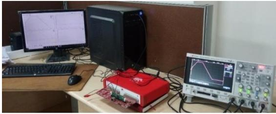
Fig. 9: HIL device and its interface
