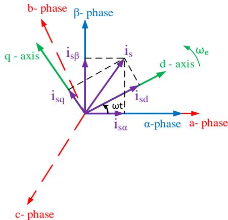
Fig. 2: Different coordinate reference-frames for SynRM
