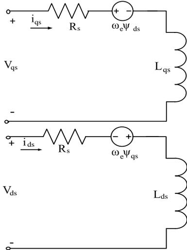
Fig. 1: Equivalent circuits of SynRM: (a) along d-axis (b) along q-axis
