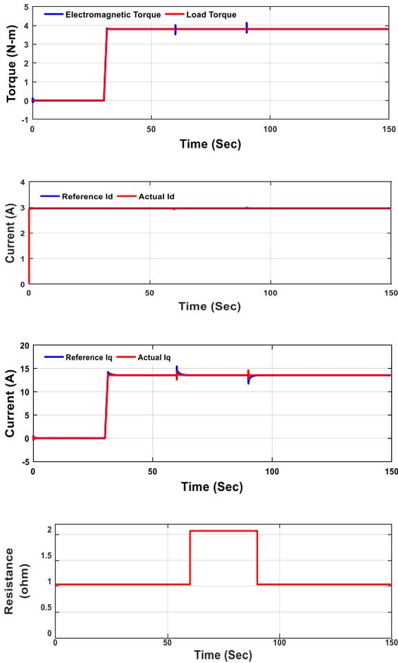
Fig. 7: Simulation results of the effect of resistance variation at low speed: (a) Command and actual Speed (b) actual and estimated speed (c) Electromagnetic torque and load torque (d) d-axis reference and actual current (e) q-axis reference and actual current, (f) Resistance variation at low speed
