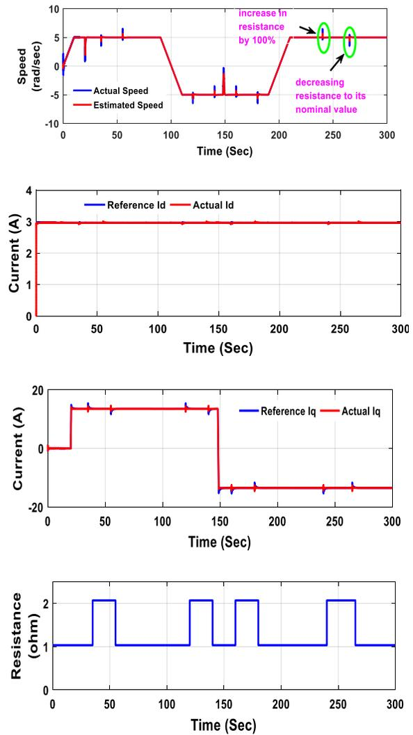
Fig. 8: Simulation results of the effect of resistance variation at low speed: (a) Command and actual Speed, (b) actual and estimated speed, (c) d-axis reference and actual current, (d) q-axis reference and actual current, (e) Resistance variation at low speed in all the four quadrant
