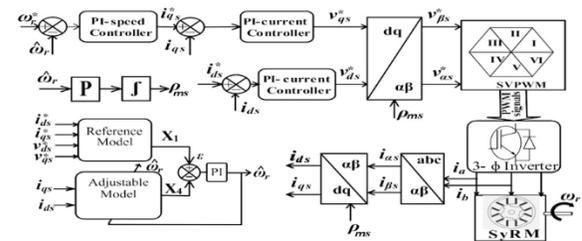
Fig 3: Vector control of SynRM drive with MRAS speed estimator
