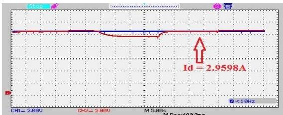
Fig. 10: HIL results of vector controlled SynRM: (a) four quadrant speed change with ramp Command (b) step change of torque (c) q- axis current (d) d-axis current
