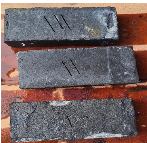
Figure 2 Moulded Bricks After 7 day curing
