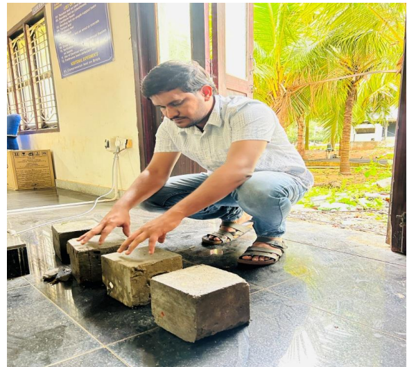
Fig. 5 Cube Specimens after Casting
