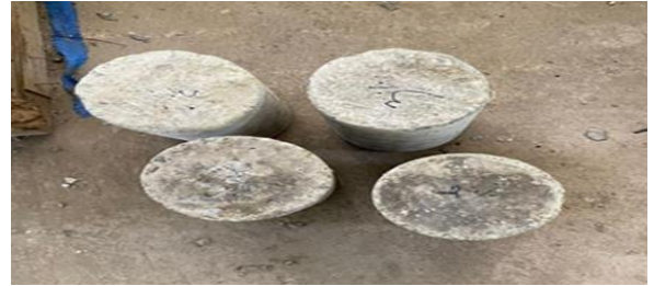
Figure I. Specimen for Compressive and Split Tensile Tests
