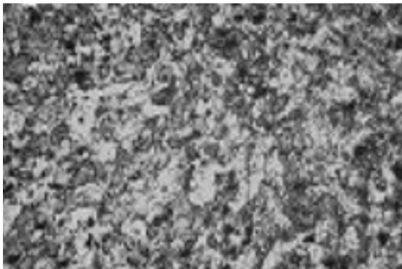
Fig5: Microstructure of AL-2014 after heat treatment From the observations we have clear that the microstructure of heat treatment alloys are changed to fine grain size to coarse grain size.
