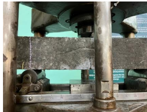
c) Testing of flexural strength of light weight concrete prism
