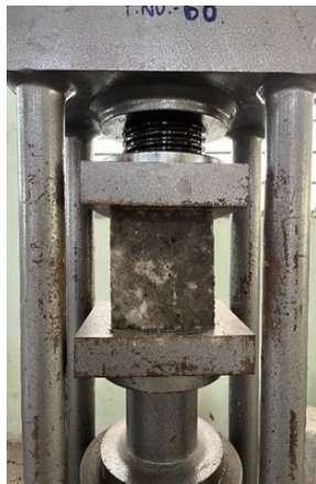
a) Testing of compression strength of light weight concrete cubes
