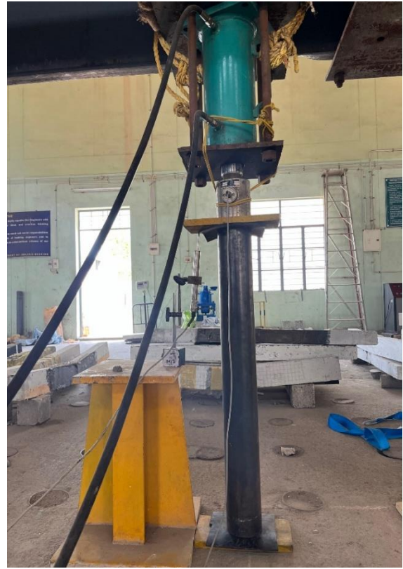
Fig 7 Test setup for CFST column under axial loading
