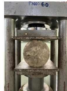
b) Testing of split tensile strength of light weight concrete cylinders
