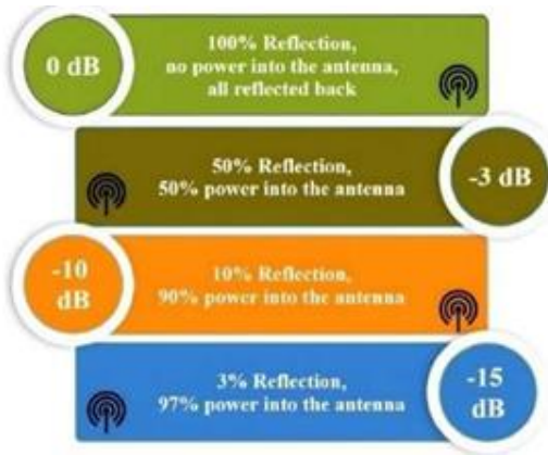
Fig.3 Importance of Antenna Return Loss
