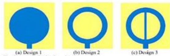
Fig.5.Iterations in designing Antenna
