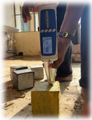
Figure 11 Rebound Hammer Test
