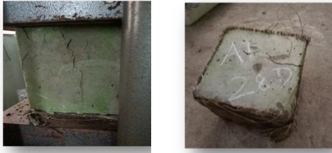
Fig.I Compression Testing on cube specimen
