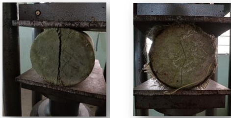
Fig.II Split tensile testing on cylinder specimen
