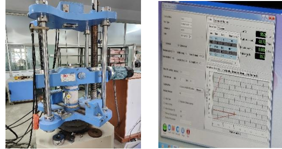
Fig 5.1 - Computerized UTM for Ferro-copper slag
