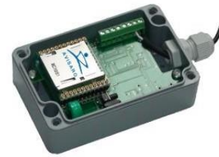
Fig 2: photography of the data logger
