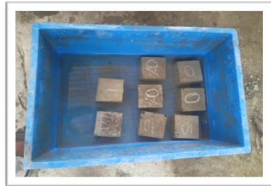
Fig 4.1 WATER ABSORPTION TEST CONDUCTED
