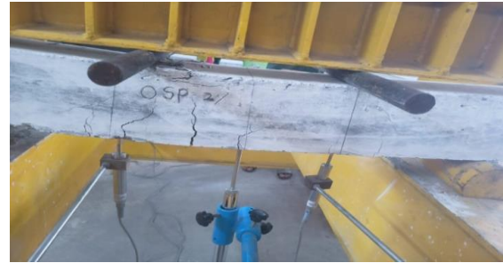
Fig 8.1.6 Failure of Beam
