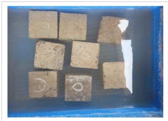
Fig 4.2.2 Acid Attack Test Conducted
