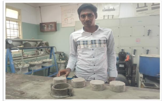
Fig 4.4.1 Sorptivity Test Specimen Conducted
