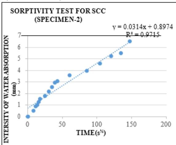
FIG 7 SORPTIVITY TEST FOR SCC (SPECIMEN-2) @ 30 DAYS RESULT CHART
