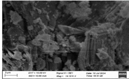
FIG 12 SEM IMAGES OF SCC-1% GF
