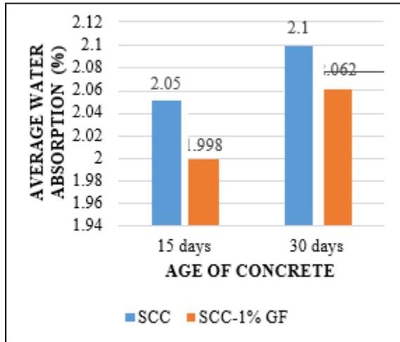
FIG 1 WATER ABSORPTION TEST GRAPH
