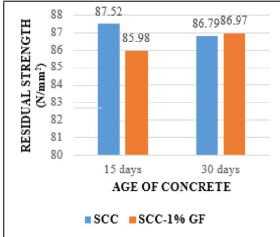
FIG 3 LOSS OF COMPRESSIVE STRENGTH AFTER ACID ATTACK (HCl) GRAPH
