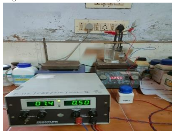
Fig 1 – Electrocoagulation reactor setup
