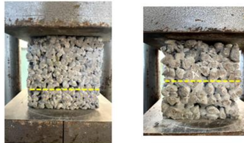
Fig 3 Compressive strength test in CTM
