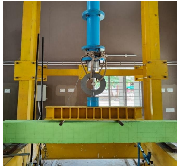
Figure.2. Flexural test on concrete specimen.
