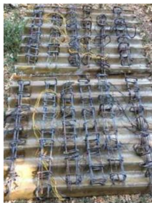
Rebars extracted after drilling
