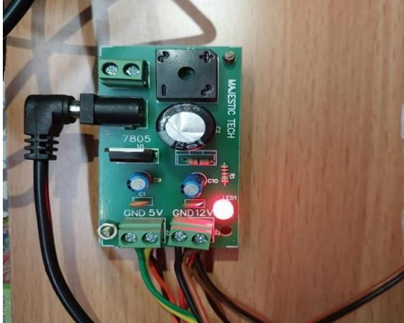
Figure 7. Power supply to convert 230v to 12v and 5v
