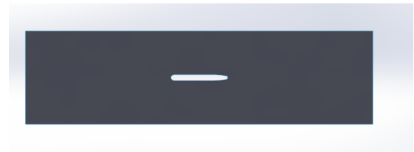
Figure 2: A torpedo-shaped underwater glider and fluid domain for numerical computation
