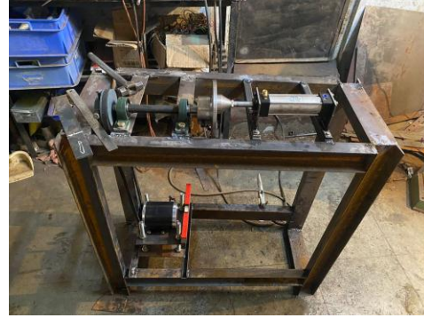
Fig: Frame of test rig- h*1*b - 900mm*750*300mm.
