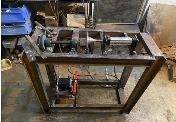
Fig: Fabrication of Brake line test rig
