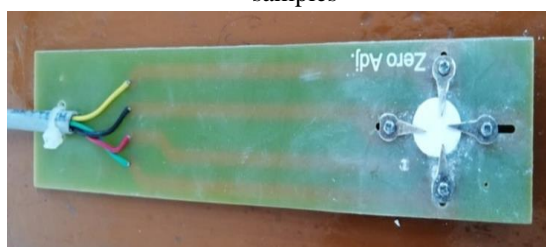
Fig. 3. The prepared sample mounted in the Hall Effect measurement circuit.
