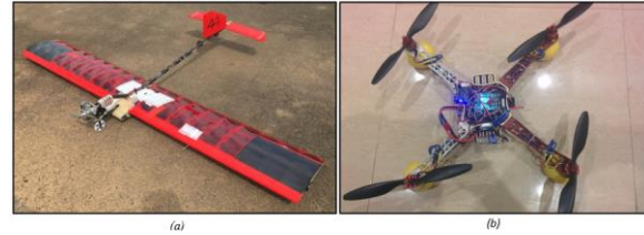
Figure 8. Comparison between (a) Fixed wing drone and (b) Rotatory motor drone
