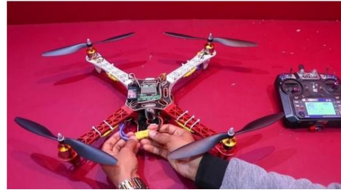
Figure 6. Connecting Lipo battery of drone to power
