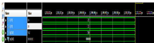
Figure 5.1 Simulation results of 8X8 Array Multiplier
