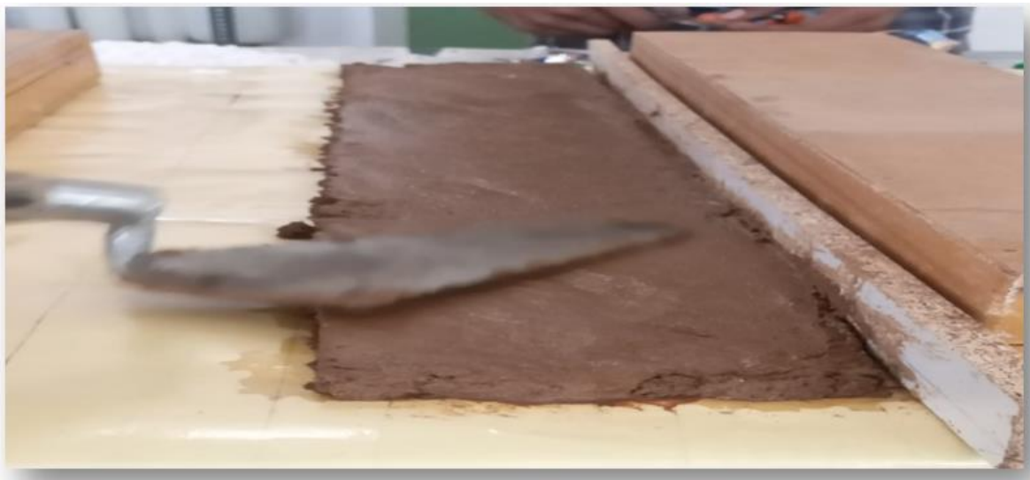
Fig 2- Layer of recycled plastic road subbase course
