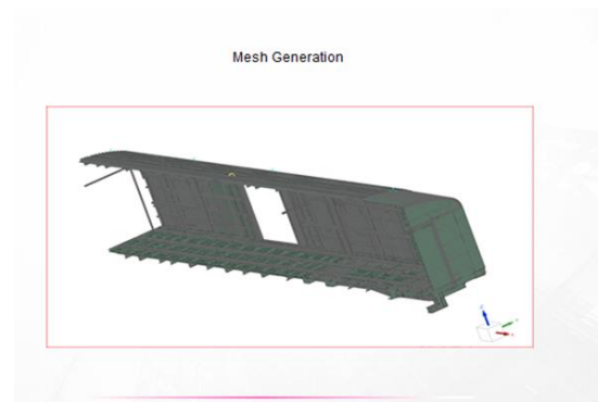
Fig 1.3: Discretized model of locomotive
