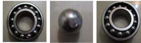
Fig 2 (a) Inner Race Crack (b) Spall on Ball (c) Outer Race Crack
