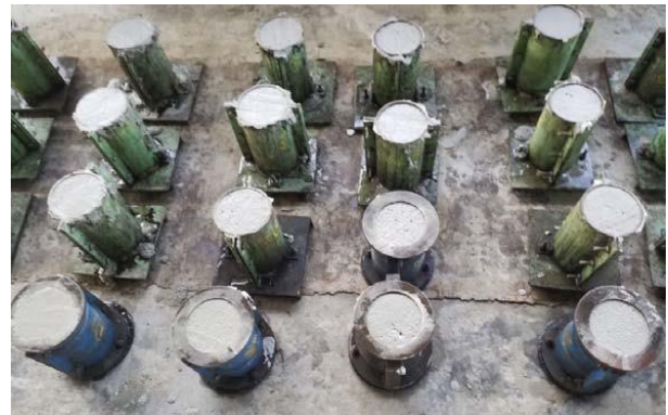
Figure 2.2 Casting of crumb rubber foamed concrete cylindrical specimens. Table 2.2 Split tensile strength results of crumb rubber foamed concrete
