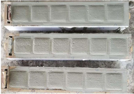
Figure 2.1 Casting of foamed concrete cube specimens with and without crumb rubber
