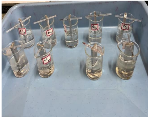
Fig. 5 corrosion test equipment and samples
