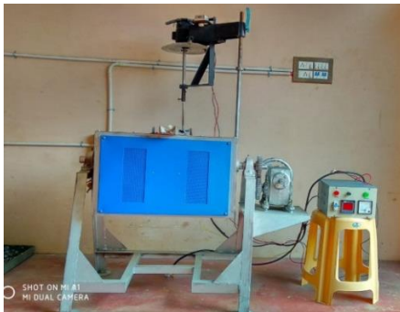
Fig. 3: Stir casting process
