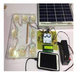
A solar piezo hybrid electric charging system integrates solar panels and piezoelectric devices to harness energy from both sunlight and mechanical stress. Solar panels convert sunlight into electrical energy, while piezoelectric materials generate electricity when subjected to pressure, such as from footsteps. The energy generated from both sources is directed to a battery through a charge controller, which manages the charging process to prevent overloading and ensures optimal energy storage.
